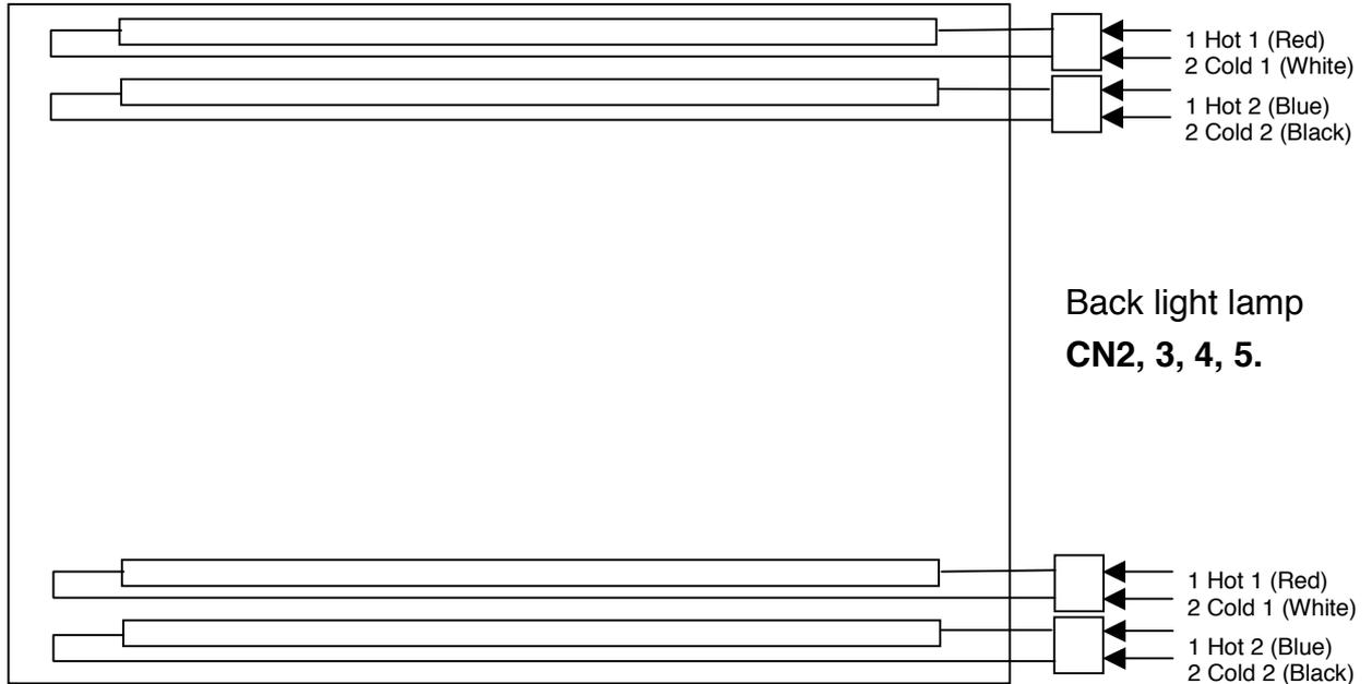
Note: The design of same polarity lamp voltage in the same lamp side of the panel is highly recommended.
