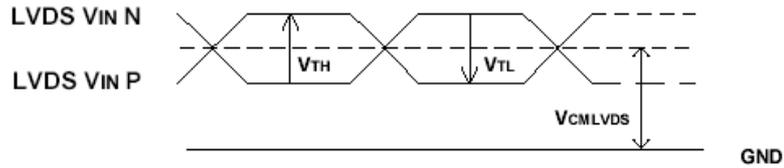
DC Timing Diagram 1: LVDS single end waveform
